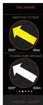
**Top: the tag for Exposure Marine's OLAS system is seen here worn on the wrist but it can equally be attached to a lifejacket, throwing line or Dan Buoy. As soon as it falls out of range of the home unit onboard an alarm triggers and the regular screen seen here flips to recovery mode (above) showing course over ground and the bearing to the incident's location**
